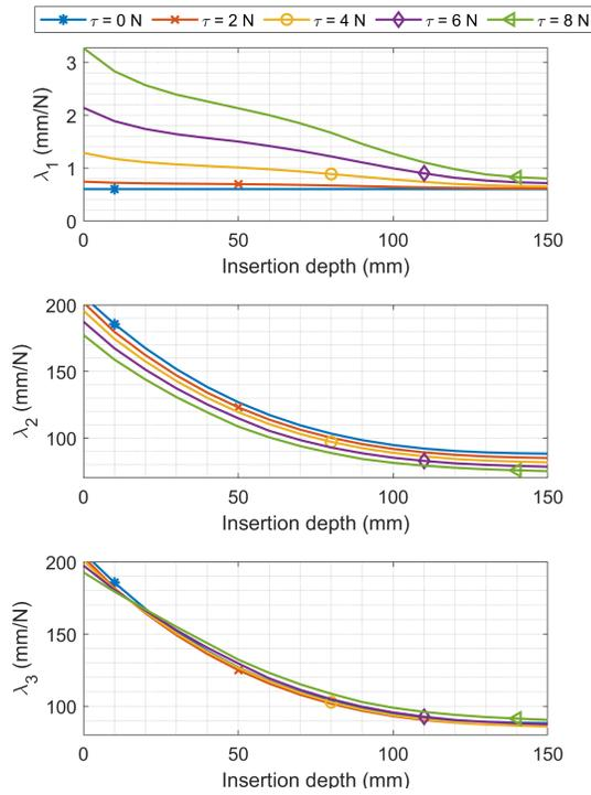
Fig. 11. The relationship between eigen value  $\lambda$  and Nitinol backbone insertion depth with various tendon tensions. The dimension of CE significantly decreases as the insertion depth increases. This shows that the stiffness of the TDCT robot tip is enhanced caused by the Nitinol backbone.
