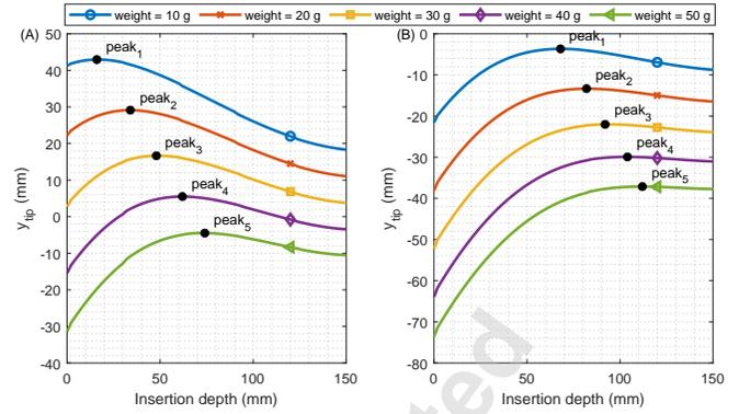
Fig. 13. Simulation studies of detailed Nitinol backbone tip position  $y_{tip}$  for various object weights and Nitinol backbone insertion depth. The peaks  $y_{tip,max}$  of each curve are highlighted with black dot marker. The tendon tension of (A) is 10 N, and the tendon tension of (B) 5 N, respectively
